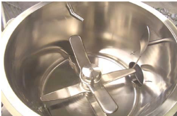
Mixing tool, material deflector, lance for addition of liquids
