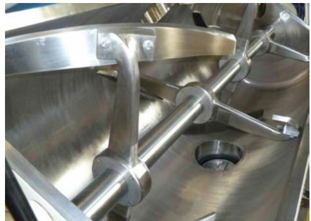
Inside view of the cooling mixer
